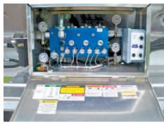
Junction boxes include wiring diagram labels inside. All utility boxes are manufactured from aluminium and all boxes are positioned for easy access.
