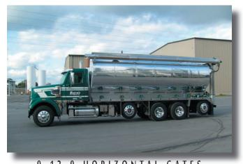
9 - 1 2 - 9 - H O R I Z O N T A L G A T E S Designed for sticky, bulky, hard-flowing materials. Allows the feed to flow without "bridging" inside the compartment.
