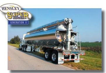
SUPER AUGER SYSTEM - 12 - 15 - 12 A Hensley Original, and our most popular auger system! Our Super Auger System can unload most feeds in 7-12 minutes!
