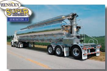
S U P E R A U G E R - H O R I Z O N T A L G A T E S Our popular gate style with a Super Auger system. Specifically designed for sticky, bulky, hard-flowing materials. Allows the feed to flow without "bridging" inside the compartment.
