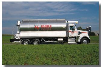
A U G E R / P N E U M A T I C U N L O A D Allows the flexibility to unload in easy-to-reach bins with an auger and the not-so-easy-to-reach bins with a pneumatic system.
