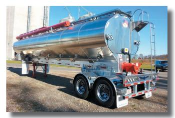
FRONT UNLOAD-9-12-9 OR 12-15-12 Front Unload trailers allow the driver to operate the augers with either an in-cab or wireless remote in full view of the truck window for easy auger placement.
