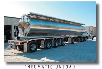
Gives the operator the ability to unload feed into places that cannot be reached with an auger system using 4" flex hoses.
