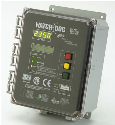
Figure 6. Typical Multi-Hazard Monitoring System for belt speed, belt misalignment, bearing temperature, plug condition, and pulley alignment for belt conveyors and bucket elevators. (Photograph courtesy of 4B Components Ltd.)
