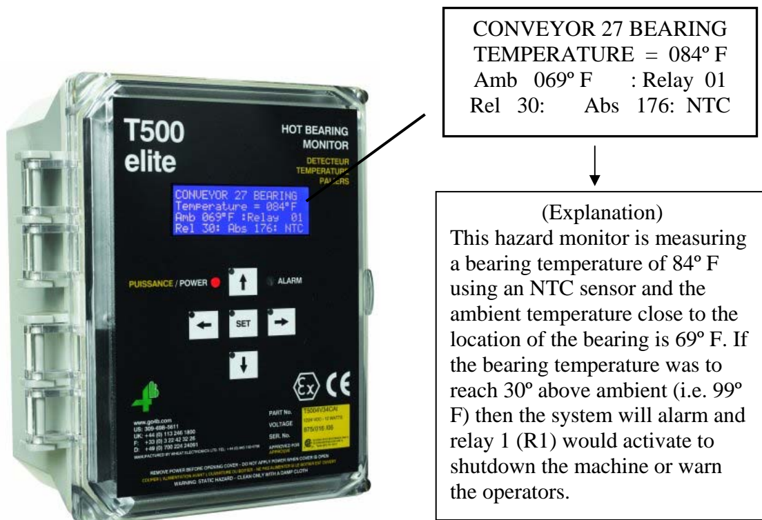
Figure 18. Continuous bearing temperature-monitoring system (Photograph courtesy of 4B Components Ltd)
