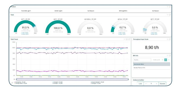
Bühler's YMS integrates data from defined scales directly into Bühler Insights, independent of the plant control system. Visualize and compare various lines against one each other. Thanks to the online data collection even those of plants in different locations. Keep track of recipe based yields over time to improve your overall mill performance.
